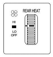
**REAR HEAT:** The thumbwheel for this system is located to the left of the audio system.
